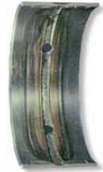
Bearing Wear caused by oil dilution
