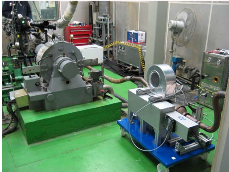
REAL-TIME OIL CONSUMPTION MEASUREMENT EQUIPMENT INSTALLED IN A TEST CELL (PROBE WITH EXHAUST FILTER AT THE BOTTOM RIGHT)
